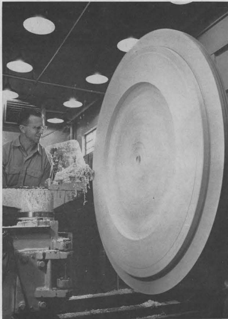
**HUGE CYLINDRICAL** pattern, 55 inches in diameter, is "turned" in a gap bed lathe by Karl McGinnis. The ring of wood will be securely glued to others and further worked as a complete unit.
